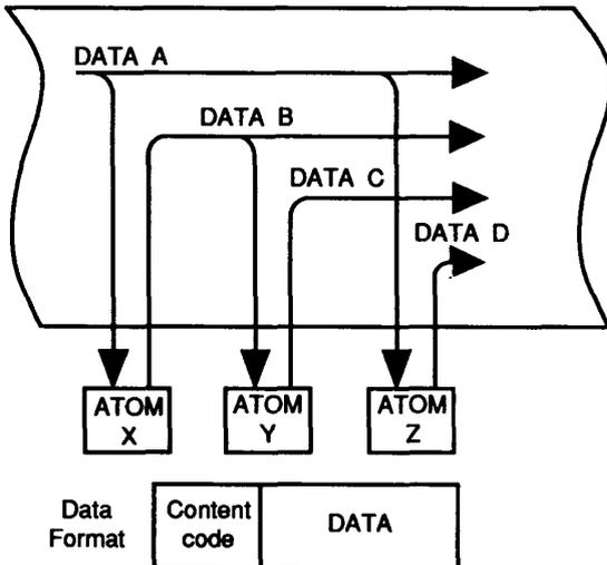
Each Atom collects the necessary DATA, execute and return the results to the Data Field.
