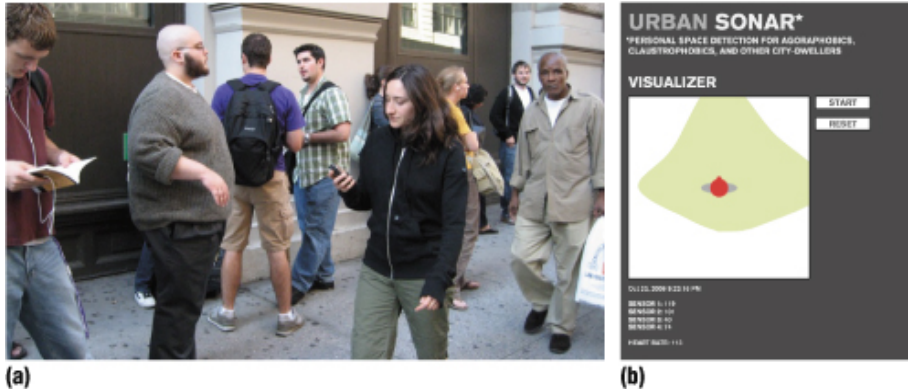
Figure 1. The Urban Sonar space monitoring system: (a) a user wears the black Urban Sonar jacket, which contains ultrasonic range finders and other electronic components; (b) the system visualizes the ebb and flow and the user’s personal space and heart rate.
