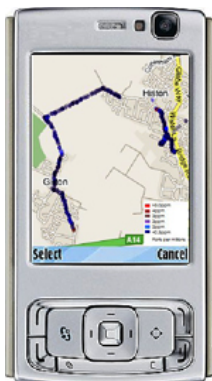
Figure 2. A screenshot of a mobile phone shows carbon monoxide data and GPS locations on Google map.
